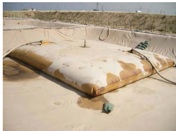
Figure 9. Example of a Class I/II and III seam leak
