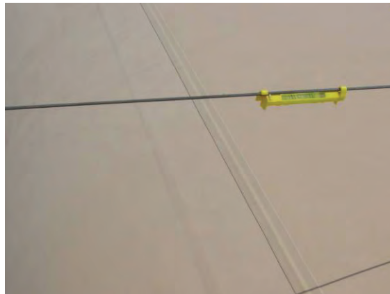
Figure 22. Line level on string.
