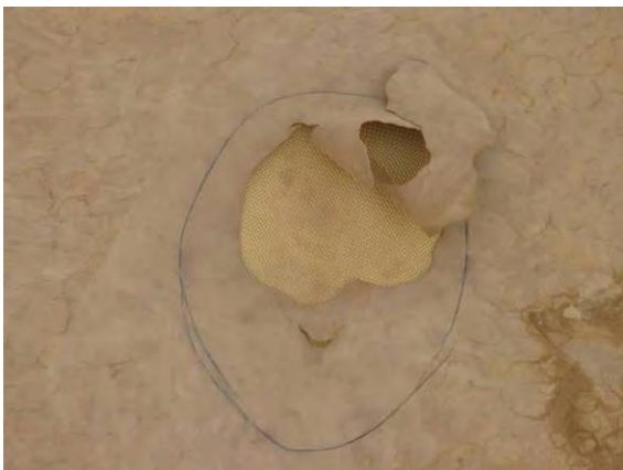
Figure 12. Example of blister in panel that ruptured
